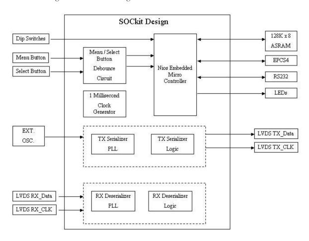
The SOCkit design can be found in the top.bdf file of the SOCkit project directory. The SOCkit designs top level module was created using Altera's schematic editor. The schematic allows the user to create graphical block representations for sub-modules. These sub-modules can then be stitched together using "wires" for connectivity. The SOCkit Design is broken into three primary design sections, which are: Nios Softcore, LVDS Serializer, and LVDS Deserializer.
